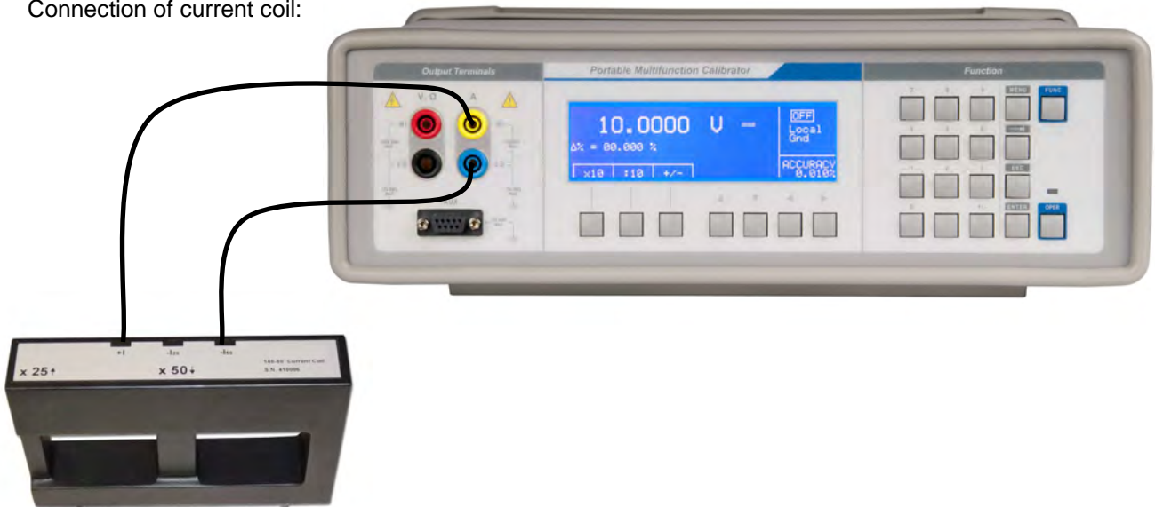
Fig. 25 Current coil connection
