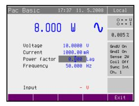
Main power value is recalculated using new set power factor and existing setting of current and voltage. The calculation is only made if active or reactive power is displayed.
