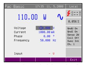
• Main power value is recalculated using new set voltage and existing setting of current and power factor.
