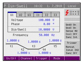
Pressing "Trigger" button starts generation of Dip/Swell shape. Generation can be started (triggered) also from input IN3. Dip/Swell shape is divided into five time periods. Length of these periods can be changed. Active period is during the generation shown in the box.
