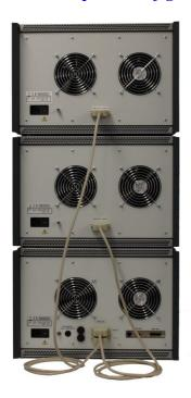
Up to two auxiliary unit MC133f(i) can be connected to the main unit MC133(i). This structure allows to generate three-phase output signal. It is possible to stack instruments. Auxiliary units are connected to the main unit by 25-wire cable (standard part of delivery). Every auxiliary unit contains calibration data. Phases are allocated according to following rules:
