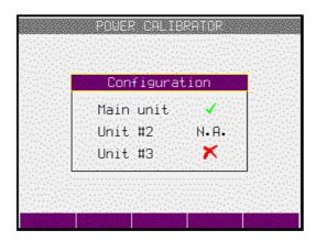
• The calibrator performs internal hardware checks for 5 seconds. Configuration of the instrument is displayed in the end of this test (connected phase channels).
