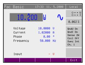
• Output power is changed by changing the value of output current.
