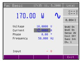
Main power value is recalculated using new set current and existing setting of voltage and power factor.
