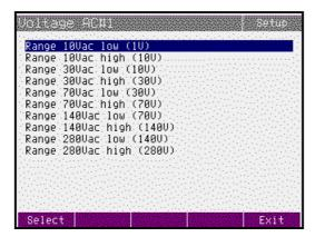
The table lists recommended calibration points. Having selected the required calibration point using Select softkey, the following data are shown.
