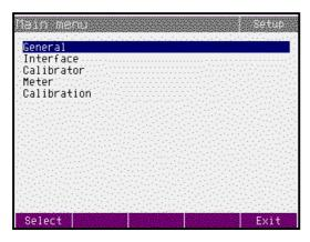
Use  $\wedge$  or  $\vee$  cursor button or the rotary knob to browse the menu options. Press "Select" softkey or press in on the rotary knob to select highlighted item. Press "Exit" softkey to leave the selected menu level.
