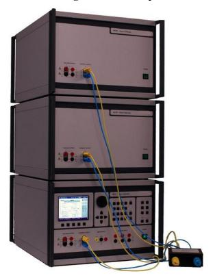
Standard part of delivery the three-phase configuration (1xMC133, 2xMC133f) is the option MC133-01. Using this adapter all current outputs are connected in parallel and the configuration can deliver up to 90 A in signle phase mode.
