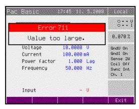
Sample error message which appears when too large value is attempted to set up is shown bellow. All error messages are displayed in the frame overlapped main screen.
