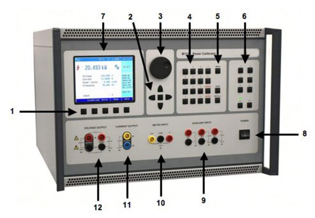
The front panel of the calibrator includes a TFT color display, control buttons and output terminals. The following picture shows the control part of the front panel.
