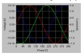
Waveform window displays amplitude, shape and phase shift for each output. Waveform window doesn't display modulation nor interharmonic components. Window displays one period of generated signal.
