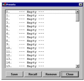
**Save** – actual parameters are stored into selected profile. There must be defined the name of the profile in case of empty profile.
