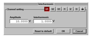
The interharmonic window allows setting of interharmonic component in the output signal. Selection of calibrator's output is described in previous paragraph (Harmonic window).
